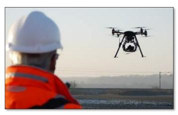
Our state-of the-art drone uses a 100MP camera to capture data to a verified sub-5mm accuracy, as well as high-resolution imagery. As one of the few companies in the UK to have Operational Safety Case (OSC) approval from the Civil Aviation Authority (CAA), we are authorised to fly in even the most congested areas of Central London, making Vogel perfect for large-scale urban regeneration projects and multi-story developments as well as highways and transport.
