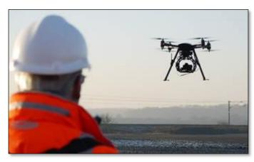
Vogel Freedom features a state-of-the-art UAV platform and a 100-megapixel camera which captures overlapping aerial images of an entire site, alongside post-processed kinematic GNSS observations and precise inertial measurement unit data. This data is then transformed into 3D data using bespoke workflows and software algorithms.
