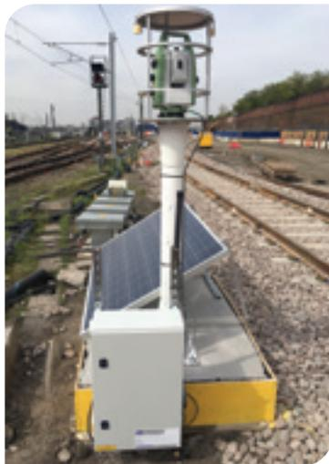
It was vital that strict Network Rail standards and measurement parameters were met and a system encompassing track prisms mounted along both running rails was installed allowing core parameters of cant, twist and displacement to be recorded. This was supplemented by structural prisms on retaining walls adjacent to a canal.
