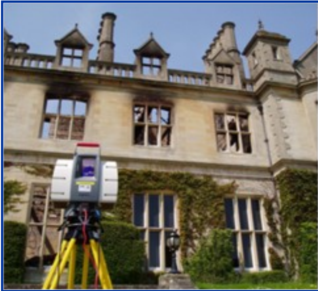
3D Laser Scanning – Post Incident Recording
