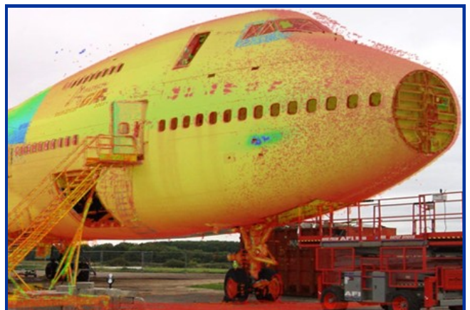
3D laser scanning – Boeing 747
